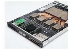
Cloud TPU v3 420 teraflops 128 GB HBM
