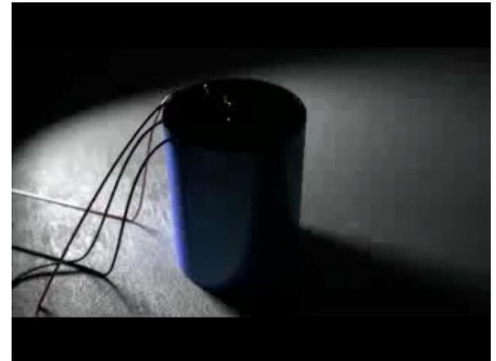
Thermal batteries provide high power density, high reliability, and a long shelf life.
