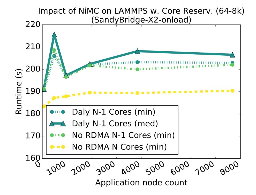
Core reservation provides a scalable solution when throttling is not enough
