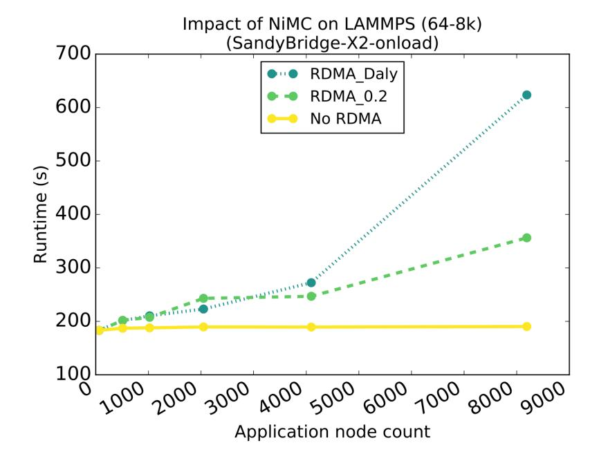
NiMC can significantly slow down single node runs by more than 100% NiMC increases LAMMPS runtime by 3X
